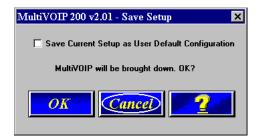
20 Select (check) Save Current Setup as User Default Configuration and click OK. The Writing Setup dialog box is displayed as the setup configuration is written to the MultiVOIP.
