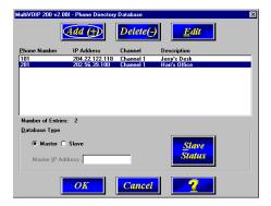
**Note:** If only Channel 1 is active, you must enter two phone numbers. The first number will be the local MultiVOIP phone number for Channel 1, and the second number will be the remote MultiVOIP phone number for Channel 1.
